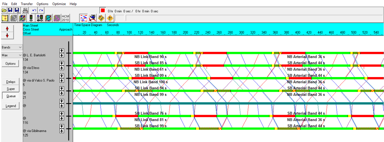
Figure 83: Time-Space diagram of Timing Plan 3 during afternoon volumes
