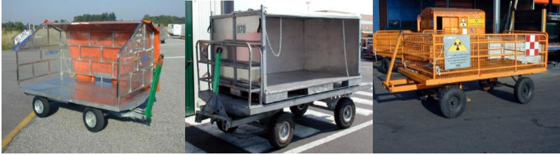
Figure 12 - Respectively carts for bulk goods, luggage and radioactive goods.
