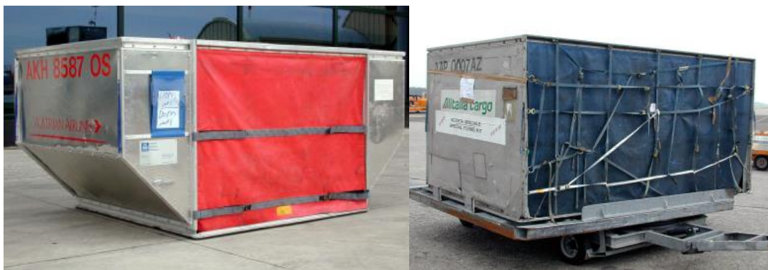
Figure 8 - Aeronautical container, on the left the AKH and on the right the AAP ULDs.
