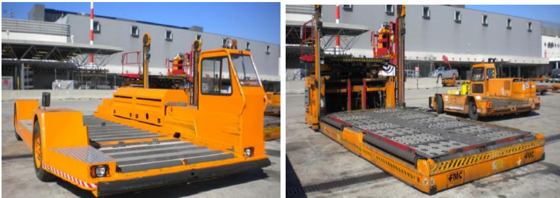
Figure 13 - On the left the transporter and on the right the cargo loader vehicles.
