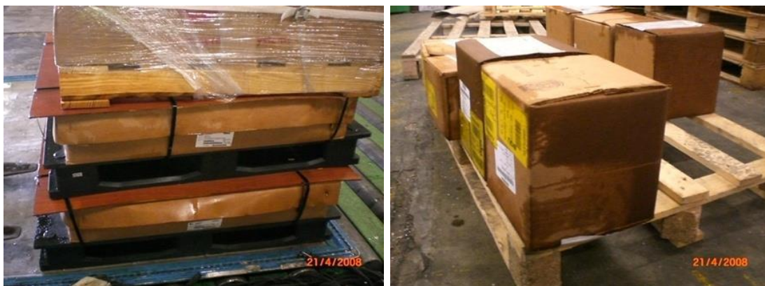
Figure 16 - Leak of fluid from the packages.
