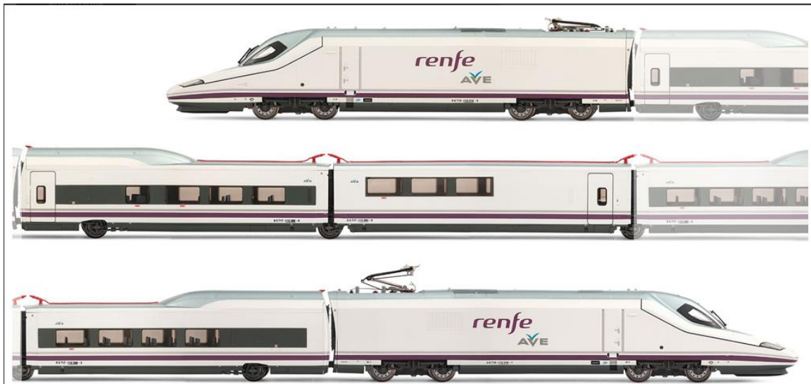
Figure 6 High-speed train with bogie type locomotives and single-axle coaches
