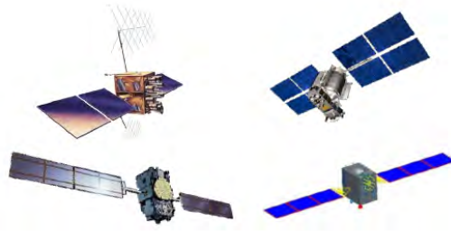
Fig. 1.2: Type of Satellites: GPS IIR-M (top left), Glonass-M (top right), Galileo IOV (bottom left) and Beidou-M (bottom right). [1]
