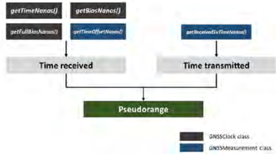
Fig. 3.3: Pseudorange generation from Android methods[9]
