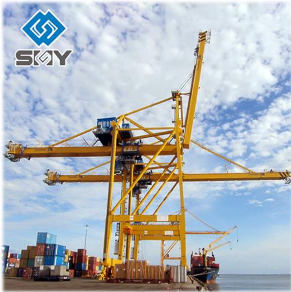
Figure 2-4. STS Crane with a box structured main boom (Henan Yuntian Crane Co.Ltd.)
