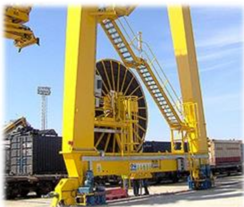
Figure 2-16. Low level mounted reel
