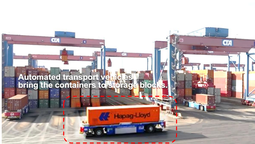
Figure 4-2. Automated container handling vehicle
