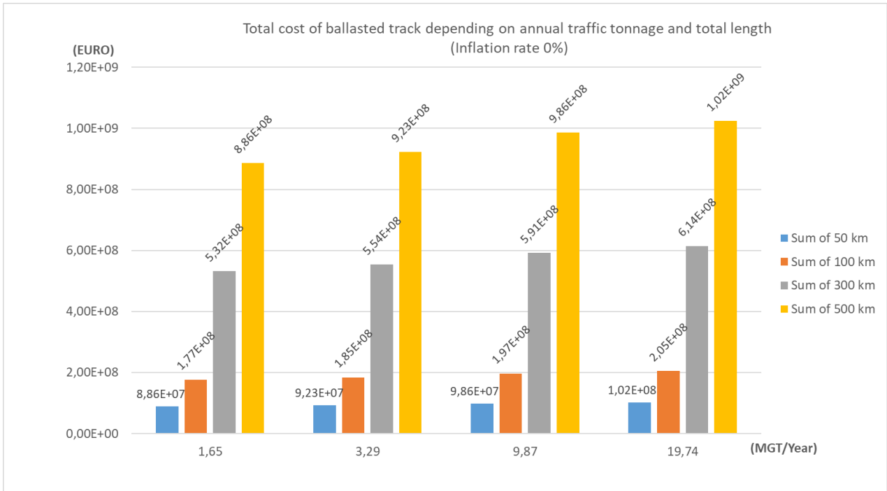
Figure 39 - LCC of ballasted track for different length and tonnage when inflation rate is 0
