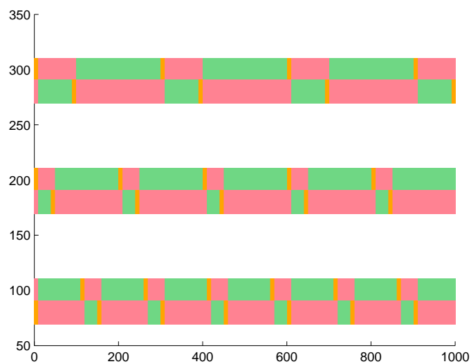
Figure 2.6: Traffic signal: succession of green, red and orange time
