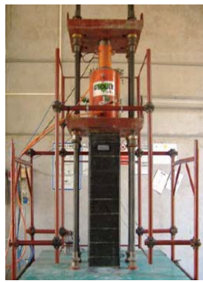
Experimental investigation on square and rectangular columns confined by CFRP.
