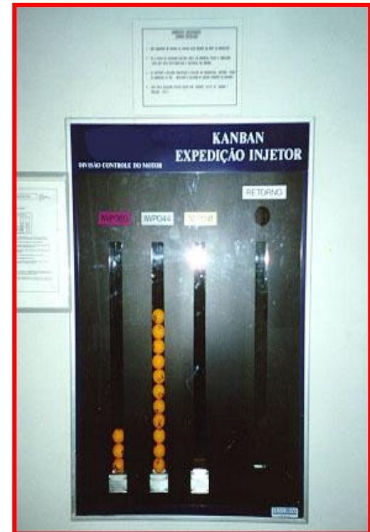
A "Ping-pong Kanban" using FIFO also indicates criticality
