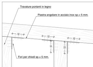
COLLEGAMENTO TRAVATURE PORTANTI-PIANTA SCALA 1:10
