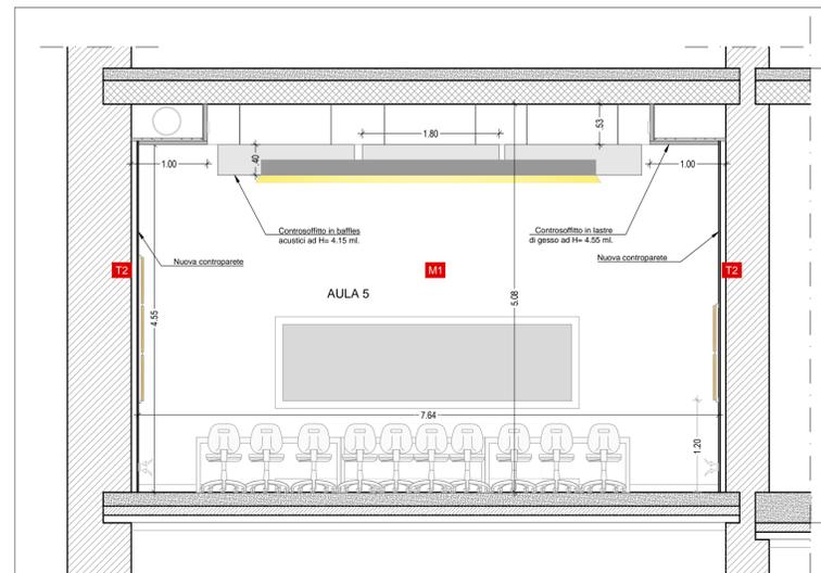
PROSPETTO-SEZIONE D-D' - SCALA 1:50
